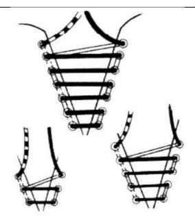
Figure 9 – Straight Across Lacing Method
